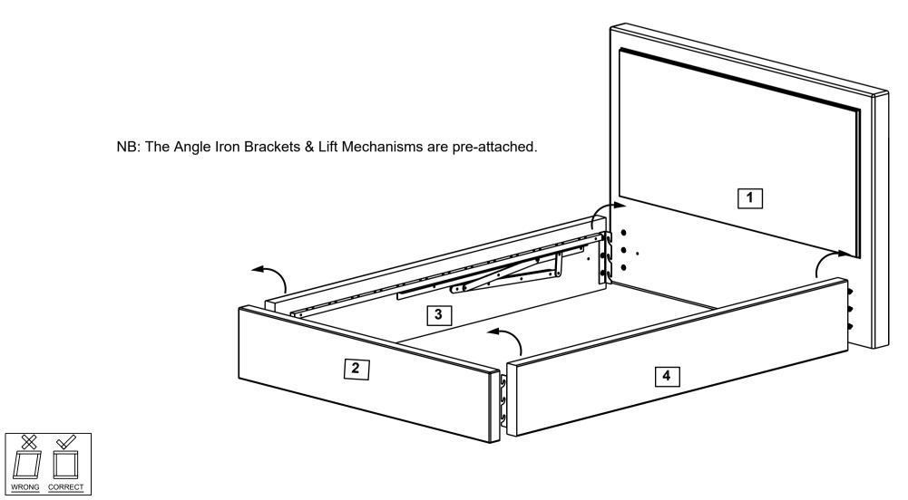
**Step 4:** Attaching the Side Rails to the Headboard & Footboard using the Angle Corner Brackets
