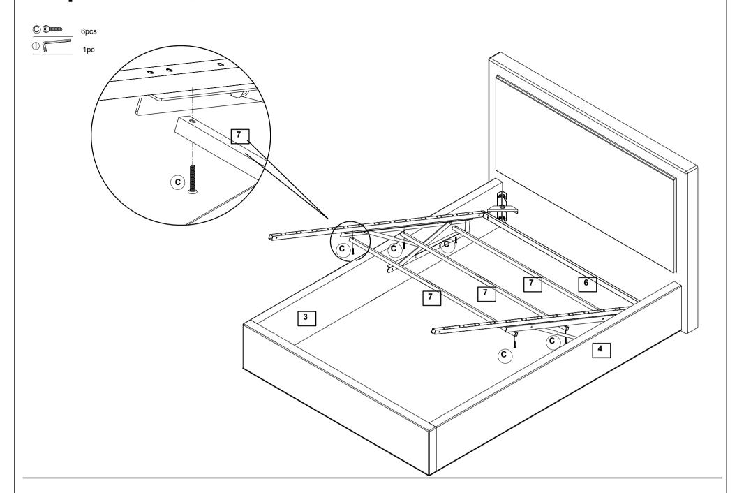
**Step 9:** Attaching the Central Support Rail to the Rear Ottoman Metal Frame
