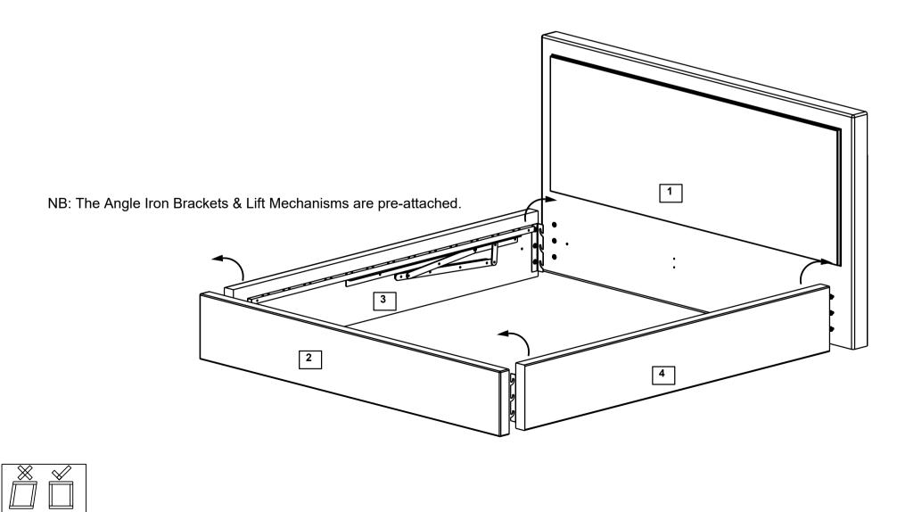
**Step 4:** Attaching the Side Rails to the Headboard & Footboard using the Angle Corner Brackets
