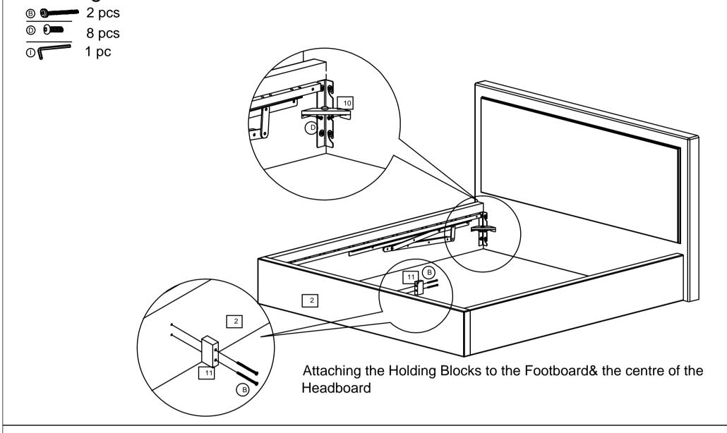
Step 5: Securing the left&Right Side Rails to the Lifting Mechanism
