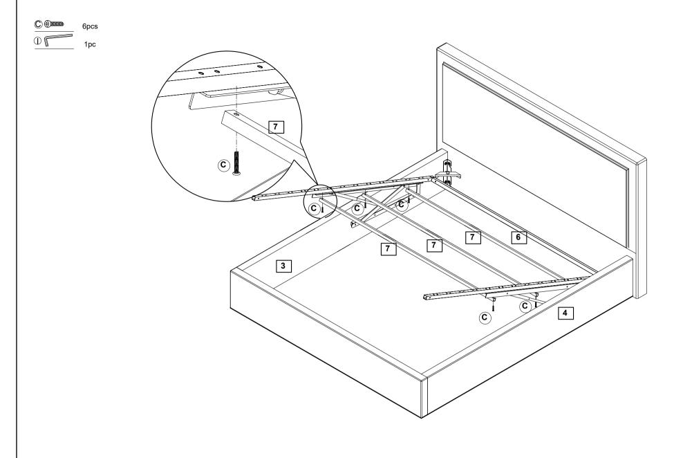
**Step 9:** Attaching the Centre Support Rail to the Rear Ottoman Metal Frame
