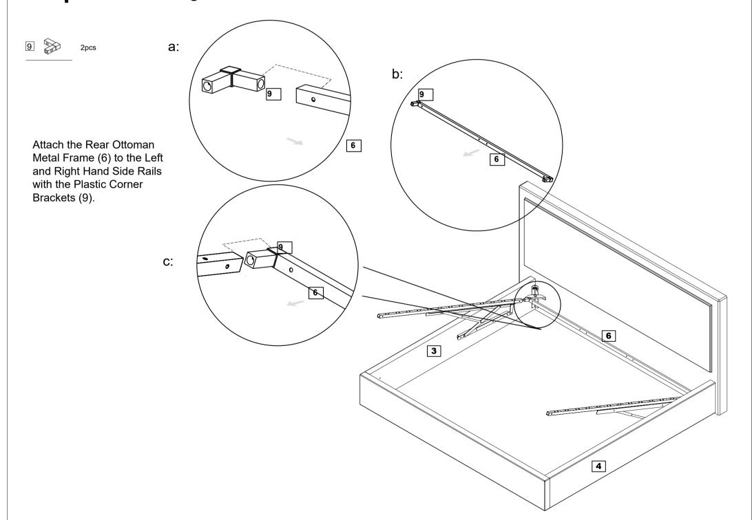
**Step 8:** Attaching the Horizontal Support Rails to the Left & Right Side Rails
