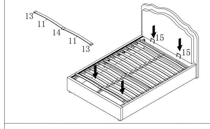
Step 15: Attaching the Strap to the Rear Ottoman Metal Frame
