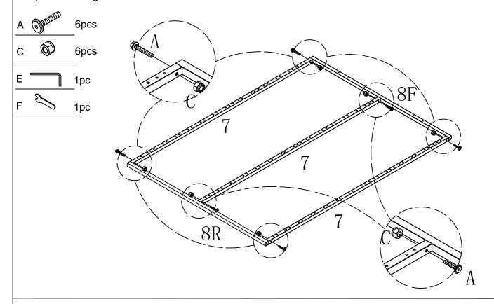
Step 9:Attaching the Side and Centre Ottoman Metal Frame to Side Rail-LH and Side Rail-RH
