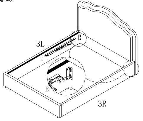
Step 5: Attaching Angle Corner Bracket to the Footboard and Side Rail-LH and Side Rail-RH. 8pcs Е 1рс 3L3R Step 6:Attaching Central Support Rail to the Side Rail-LH and Side Rail-RH.
