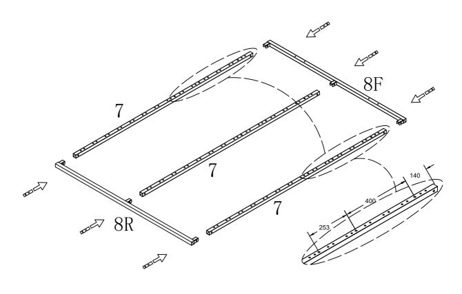
Step 8: Attaching the Side and Centre Ottoman Metal Frame to the Front/Rear Ottoman Metal Frame
