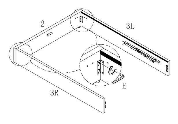
Step 4:Attaching the Side Rail-LH and Side Rail-RH to the Headboard, hook the Connector onto the screws before tigihtening fully.
