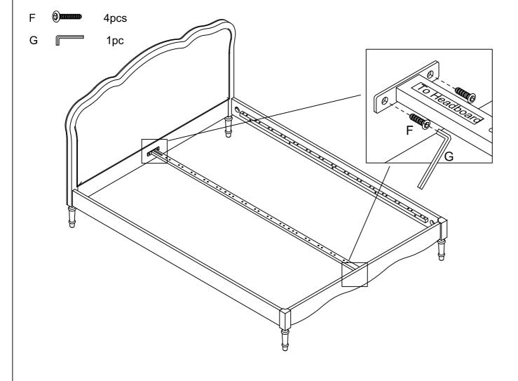
Step 5: Attaching the Slat Caps & Slats to the Bed Frame
