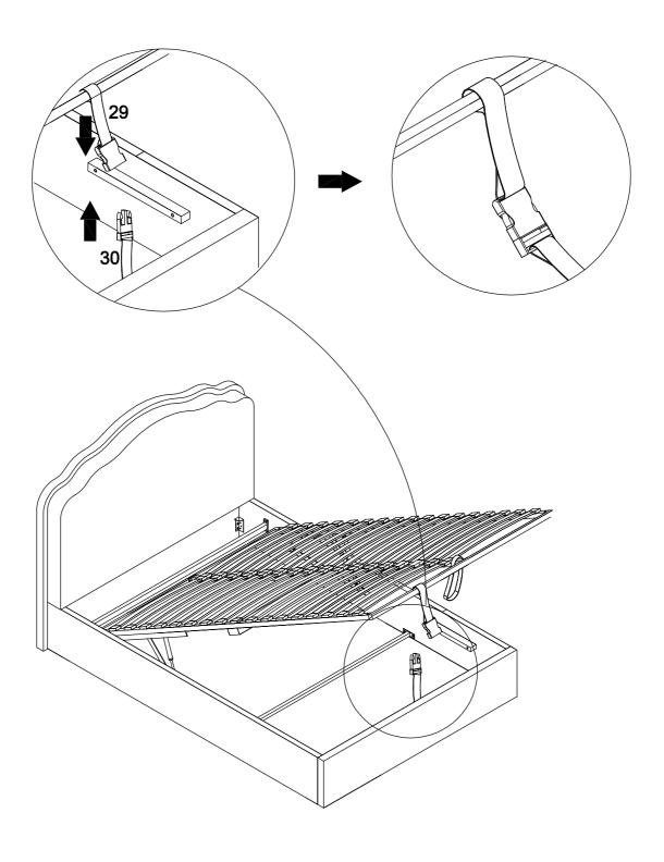
Warning: Lock the buckle after close of gas-lift to avoid opening automatically.
