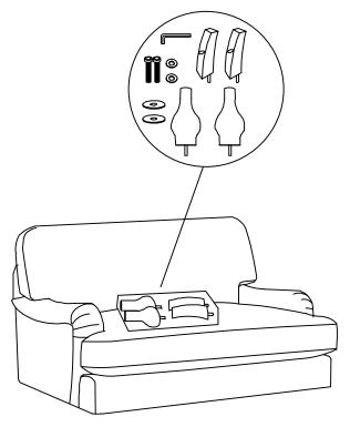
Step 2 Fasten the front legs and affix the rear legs as shown in the above diagram using the bolts supplied.
