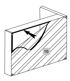
With an assistant, carefully lift both the Headboard &Footboard at the same time, do not let the bed frame twist. Lift and turn the bed frame on its side holding the bed upright for safety. Attach the Fabric Base (16) to bottom of the Side Rails, Headboard & Footboard with the velcro tape. Ensure the fabric is fixed evenly all round.
