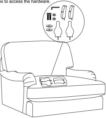
Step 2 Fasten the front legs and affix the rear legs as shown in the above diagram using the bolts supplied.
