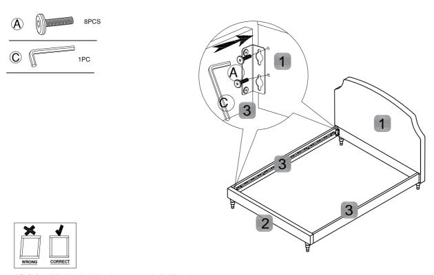
NB: Before tightening the bolts, please ensure the bed frame is square
