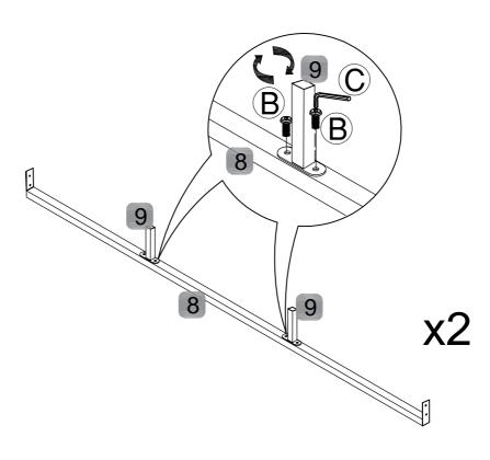
Step 4: Attaching the Central Support Rail to the Headboard & Footboard
