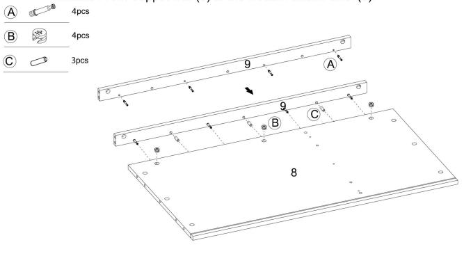
Step 9: Attach the Bottom Shelf Panel (8) to the Frame.
