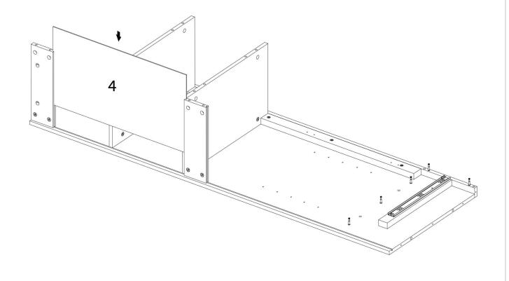
Step 5: Attach the Cam Bolt to the Middle Panel (5).
