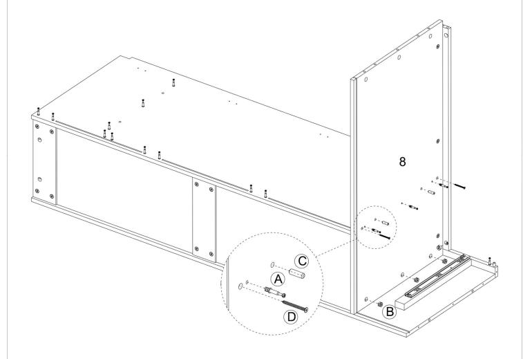
Step12: Attach the Cam Bolt to the Middle Front Support Bar(20), then attach the Middle Front Suppot Bar(20) to the Bottom Shelf Panel (12).
