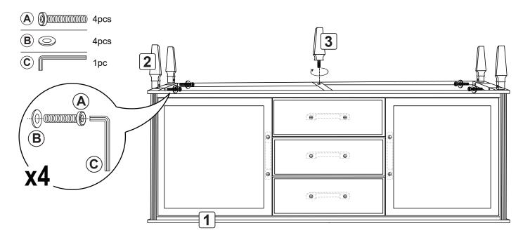
**Step 2:** Handles are pre-attached inside the drawers and doors. Disassemble the pre-attached handle and reattach as shown in the figure.
