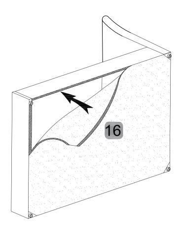
With an assistant, carefully lift both the Headboard & Footboard at the same time, do not let the bed frame twist. Lift and turn the bed frame on its side holding the bed upright for safety. Attach the Fabric Base (16) to bottom of the Side Rails, Headboard & Footboard with the velcro tape. Ensure the fabric is fixed evenly all round.
