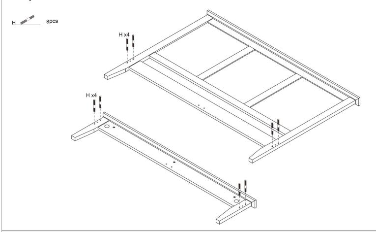
**Step 7:** Attach the Central Support Legs and Corner Brackets to the Central Support Rail.
