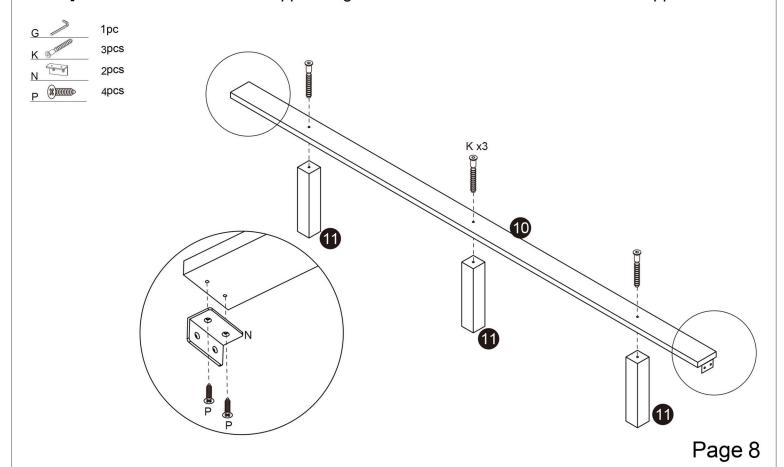
**Step 8:** Attach the Side Rails and Central Support Rail to the Headboard and Footboard.
