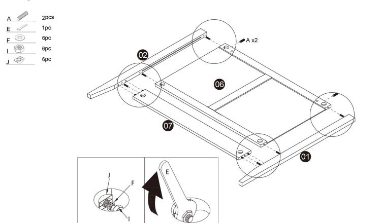
**Step 3:** Attach the Top Panel to the Back Panel.
