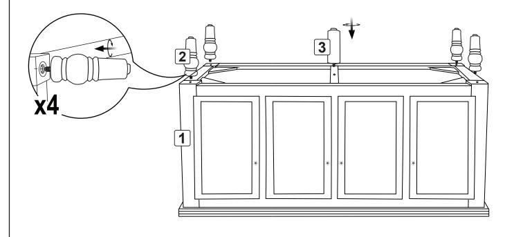
**Step 2:** Door handles are pre-assembled reversely. Disassemble the handle and re-attach as shown in the figure.
