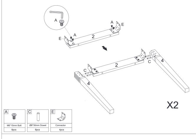
2. Attach bolts to the Frame. The bolts are tightened to 80% of their maximum torque.
