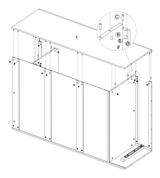
Step 14: Attach Lower Back Panels (18) to the Frame and attach the Dowel (C) to the Frame. **©** 6pcs
