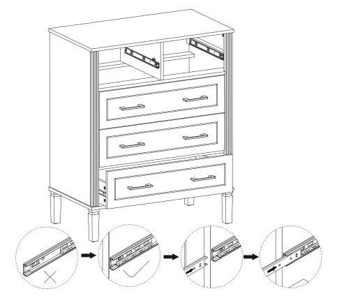
19. Attach the plastic buckles on back. Before securing them, manually adjust the frame to ensure the drawers are properly aligned, even, and parallel.
