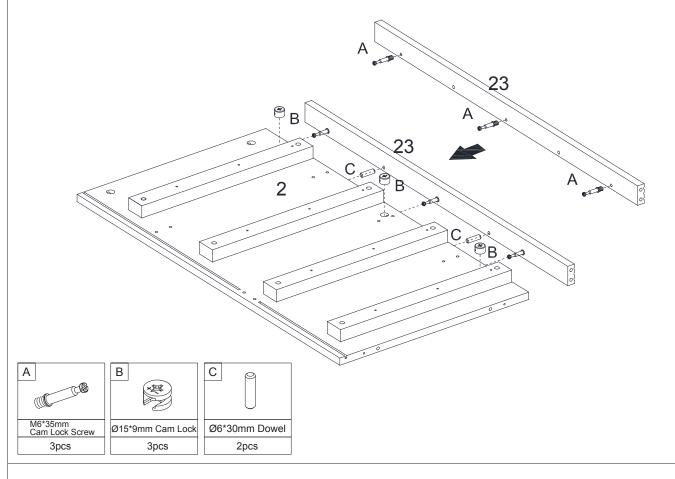
2. Attach fitting and Slide Rail to Right Side Panel (2).
