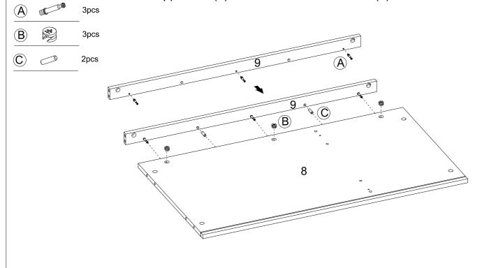
Step 16: Attach the Bottom Shelf Panel (8) to the Frame.
