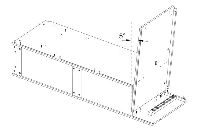
Step 18: Attach the Slide Rail to the Bottom Middle Panel (38).
