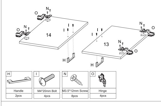
16. Attach the Doors (13,14) to the Frame. Slide the drawers into the Frame. The Centre Leg is adjustable if necessary.
