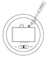
Step 1: Use a screwdriver to loosen the screw and open the battery case cover.
