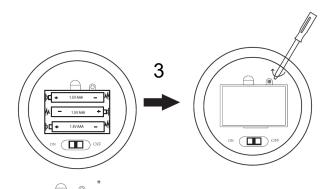
Step 3:Close the battery case cover and tighten the screw. Then turn the switch to "ON" position and light up.
