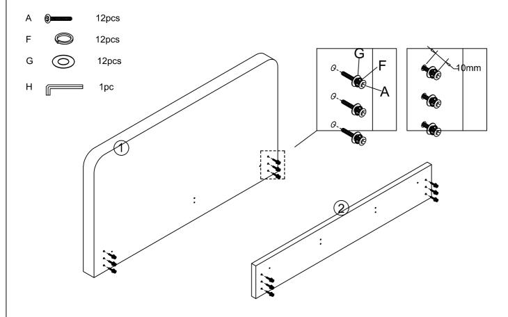
**Step** 3: Attaching the Left & Right Side Rails to the Headboard &Footboard 1pc NB: The Angle Iron Brackets & Lift Mechanisms are pre-attached. NB: Before tightening the bolts, please ensure the bed frame is square Step 4: Attaching the Side Rails to the Headboard & Footboard using the **Angle Corner Brackets** 6pcs 8pcs 1pc **⊚**D **\$** B
