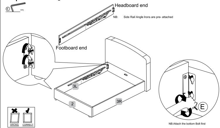
NB: Before tightening the bolts, please ensure the bed frame is square
