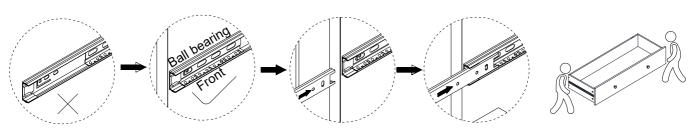
The assembly of the large drawer requires twopeople to align the slide rails synchronously
