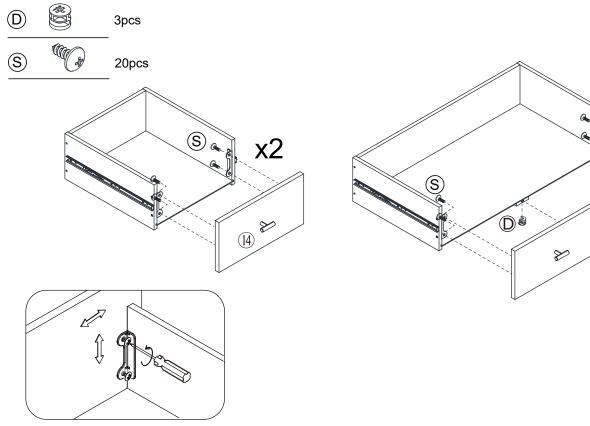
Adjust drawer sides' position by turning Screw (S) clockwise or counterclockwise as necessary.
