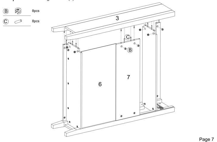
Step 7: Insert Upper Back Panel (8) to the frame.
