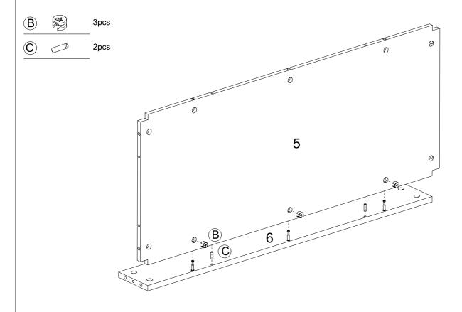
Step 5: Attach another Upper Panel (6) to Shelf Panel (5).  $\bigcirc$ 3pcs **(C)** 2pcs 6 O- **©**  $^{\text{O}} \, \, \text{\textcircled{B}}$ 5 Step 6: Attach cam bolts and felt mat to Left Panel (1) and Right Panel (2).
