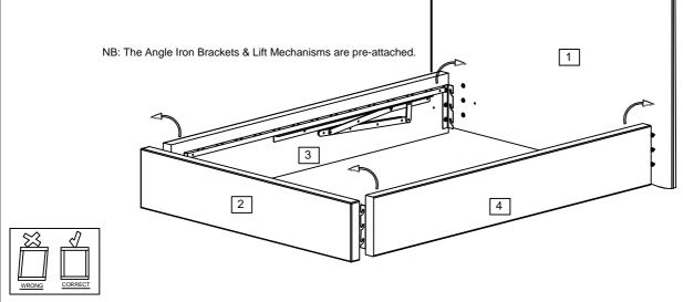
NB: Before tightening the bolts, please ensure the bed frame is square
