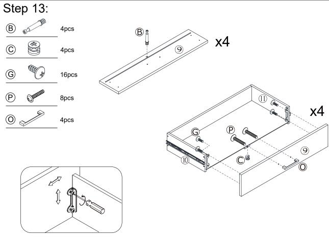
Adjust drawer sides' position by turning Screw (G) clockwise or counterclockwise as necessary.
