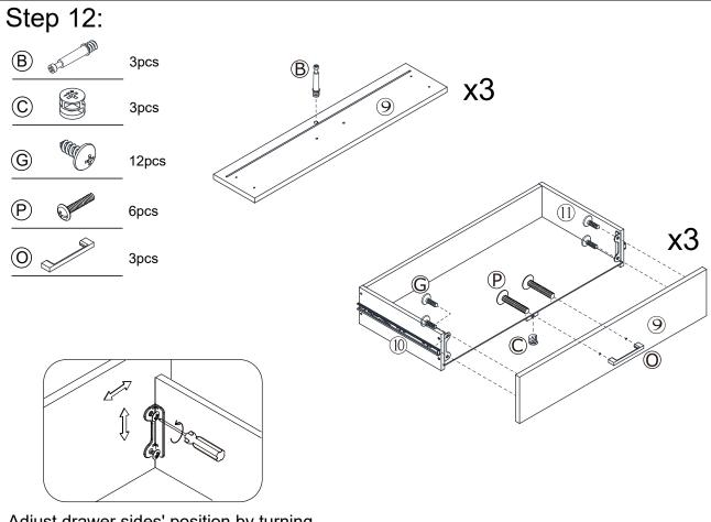
Adjust drawer sides' position by turning Screw (G) clockwise or counterclockwise as necessary.
