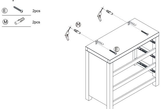
Before applying the bracket to the wall, check pipes and cables that may be hidden behind.
