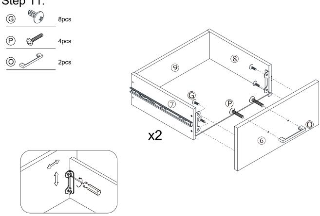
Adjust drawer sides' position by turning Screw (G) clockwise or counterclockwise as necessary.
