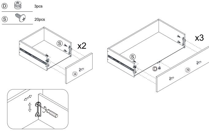
Adjust drawer sides' position by turning Screw (S) clockwise or counterclockwise as necessary.
