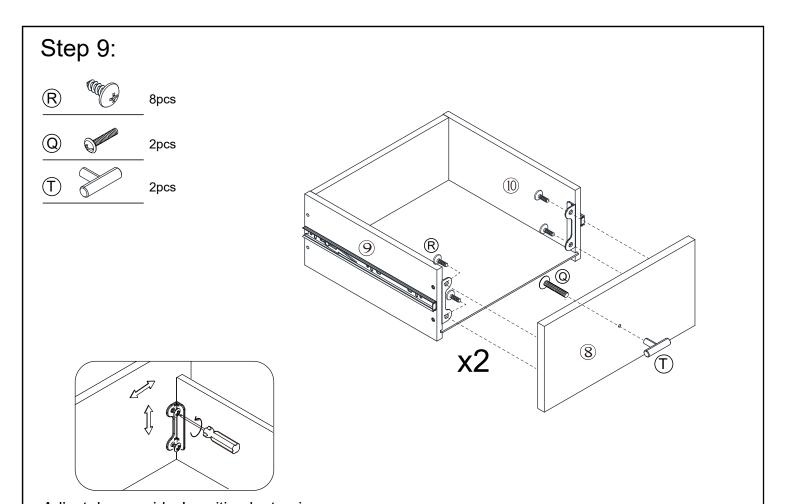
Adjust drawer sides' position by turning Screw (R) clockwise or counterclockwise as necessary.
