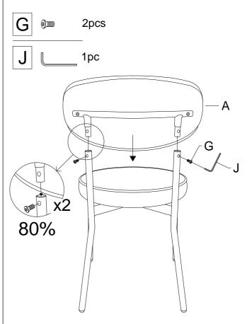
Step 4: Put the assembled chair onto a flat base and then fully tighten all bolts.
