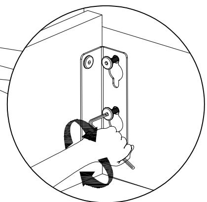
NB: Attach the bottom Bolt first
