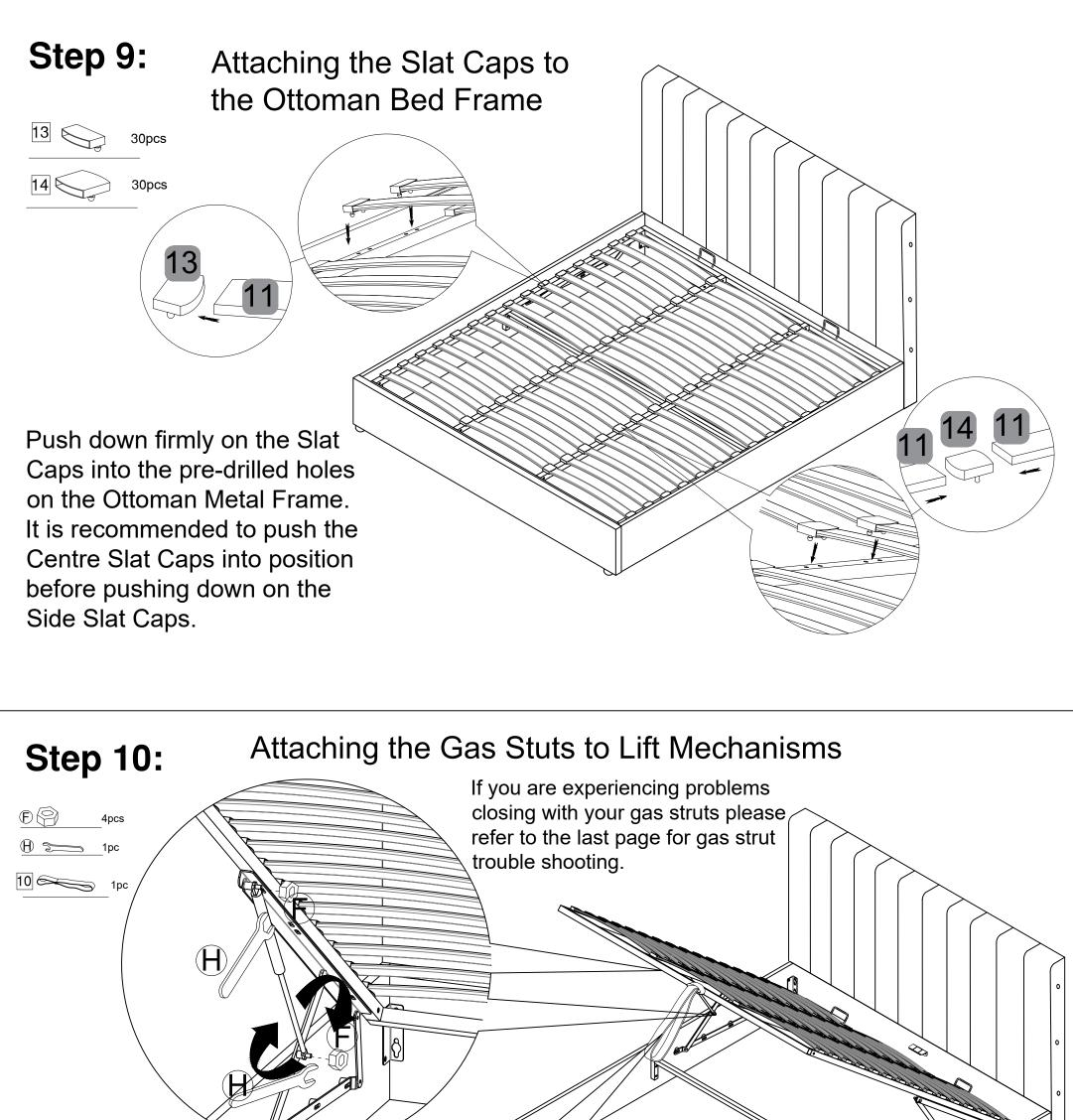
Attach the Strap (10) to the Center Ottoman Metal Frame, at the Footboard end.
