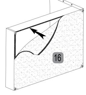
With an assistant, carefully lift both the Headboard & Footboard at the same time, do not let the bed frame twist. Lift and turn the bed frame on its side holding the bed upright for safety. Attach the Fabric Base (16) to bottom of the Side Rails, Headboard & Footboard with the velcro tape. Ensure the fabric is fixed evenly all round.
