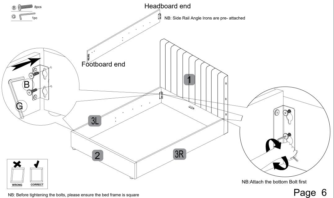
NB: Before tightening the bolts, please ensure the bed frame is square
