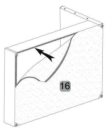
With an assistant, carefully lift both the Headboard & Footboard at the same time, do not let the bed frame twist. Lift and turn the bed frame on its side holding the bed upright for safety. Attach the Fabric Base (16) to bottom of the Side Rails, Headboard & Footboard with the velcro tape. Ensure the fabric is fixed evenly all round.
