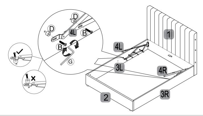
**Step 5:** Attaching the Central Support Rail & Angle Corner Brackets
