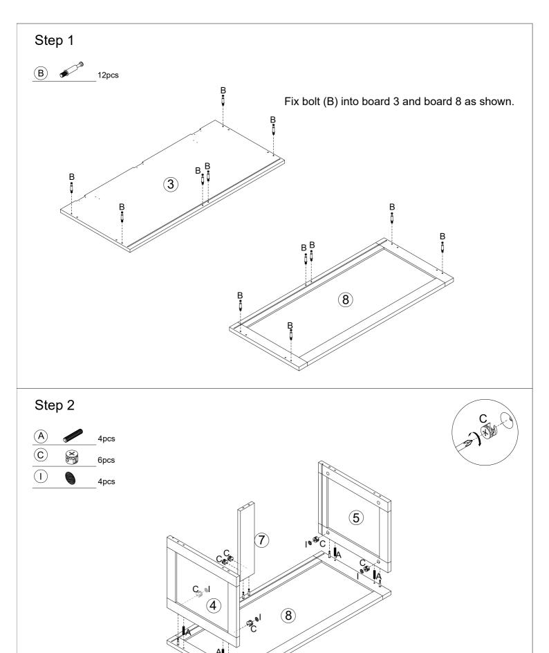
Attach board 4 and board 5 to board 8 with wooden dowel (A) first then put cam (C) into board 4 and board 5 then turn clockwise to tighten, stick the cam hole with sticker(I) as shown.
