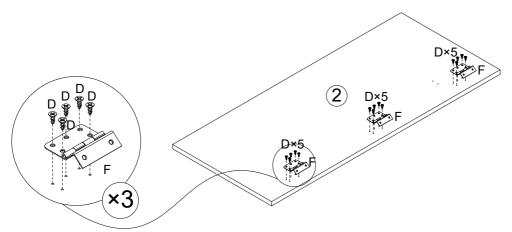
Fix hinge (F) into board 2 with screw (D) as shown.
