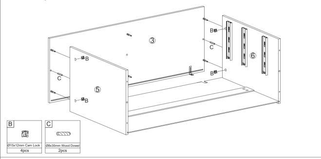
6. Attach middle panel to the top, fix with cam lock and cover with covers.
