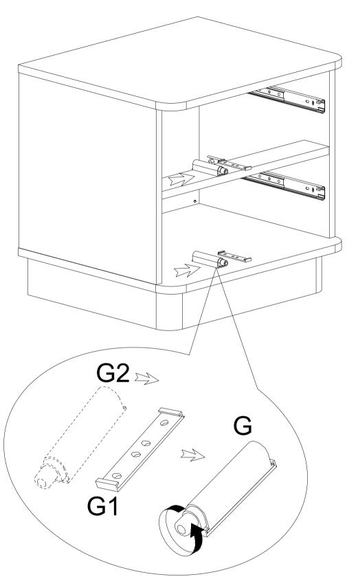
After assembling G1 and G2 into G,rotate the front of G counterclockwise by 3mm.
