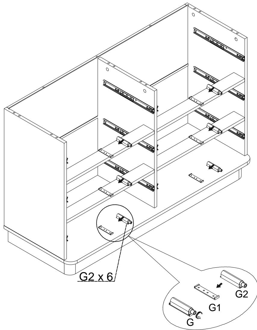
After assembling G1 and G2 into G, rotate the front of G counterclockwise by 3mm
