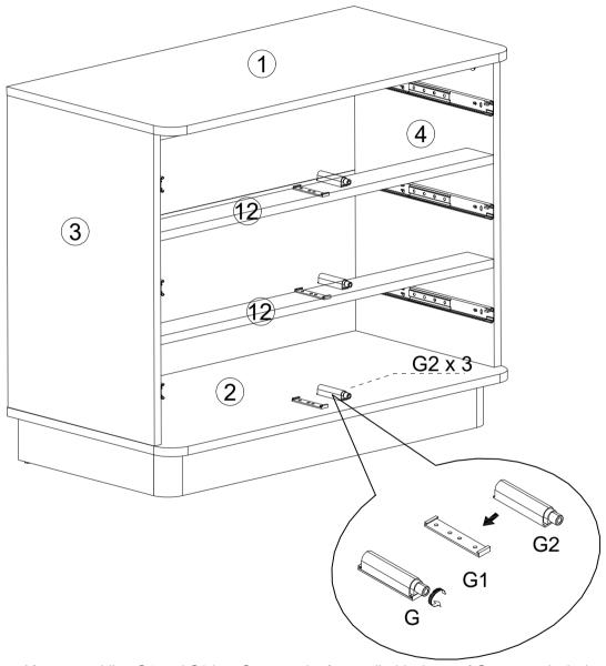
After assembling G1 and G2 into G, rotate the front cylindrical part of G counterclockwise by 3mm.
