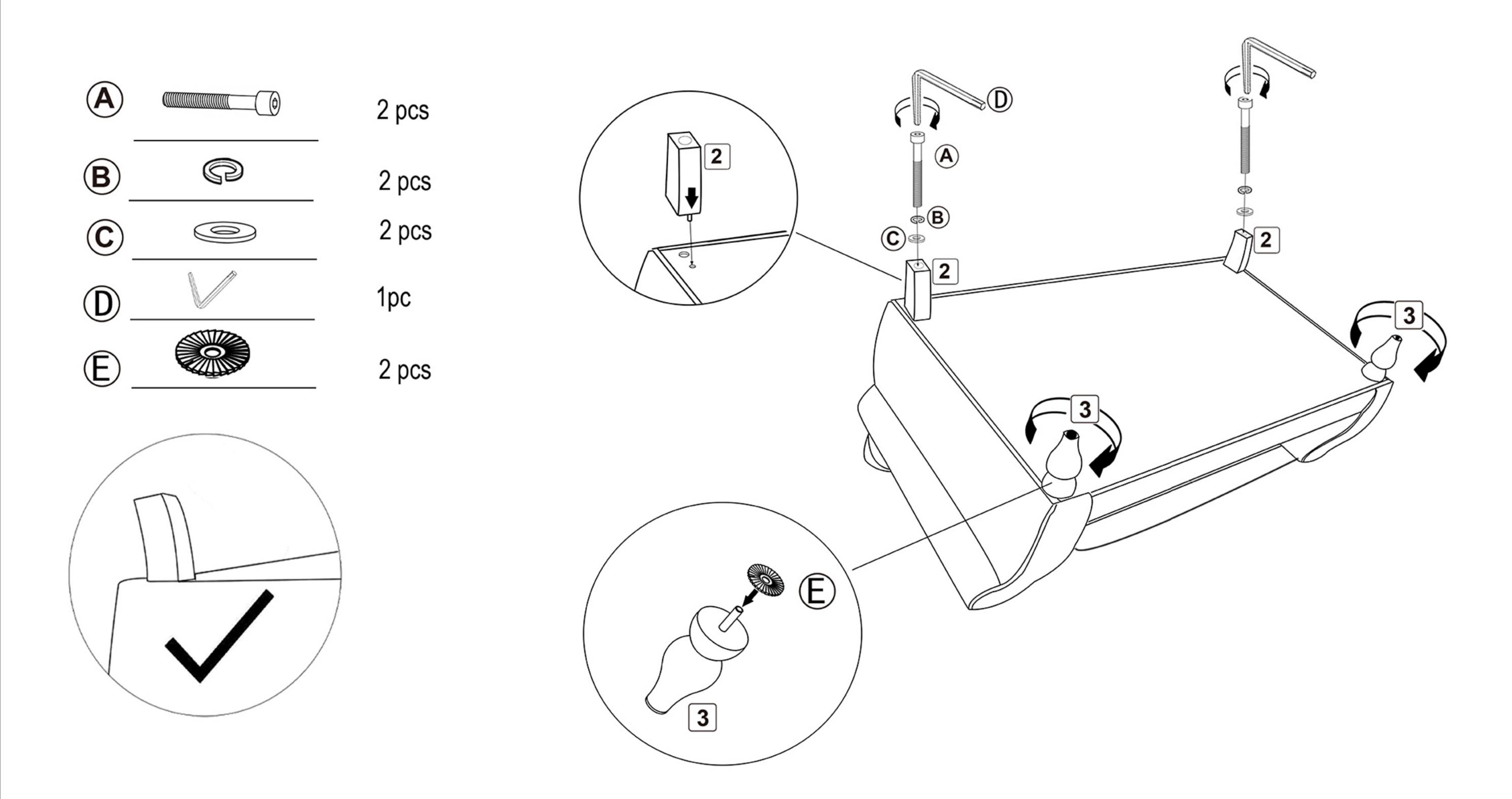
Step 3: Apply the felt pads on the bottom of the back feet.
