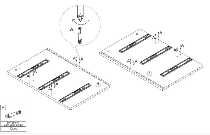
Step 2. Assemble the left and right side panels with horizontal bars.
