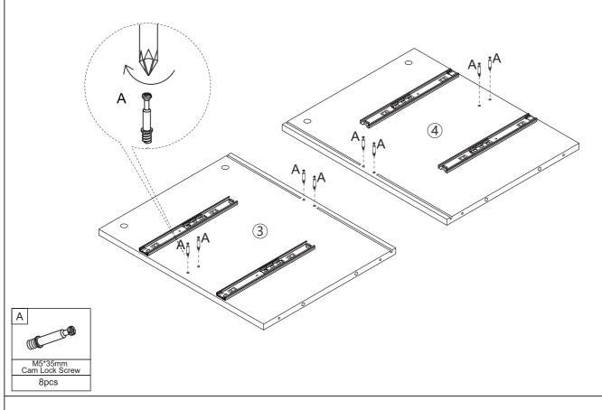
Step 2. Assemble the left and right side panels with horizontal bars.
