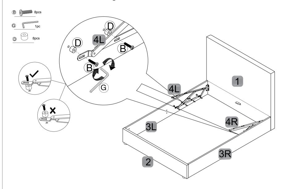
Step 4: Attaching the Central Support Rail & Angle Corner Brackets
