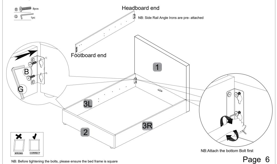
**Step 3:** Attaching the Side Rails & Lift Mechanisms
