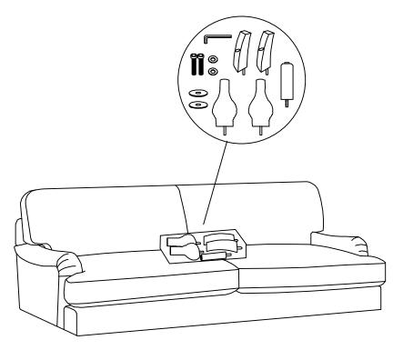
Step 2 Fasten the front legs and middle support leg and affix the rear legs as shown in the above diagram using the bolts supplied.
