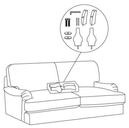
Step 2 Fasten the front legs and affix the rear legs as shown in the above diagram using the bolts supplied.
