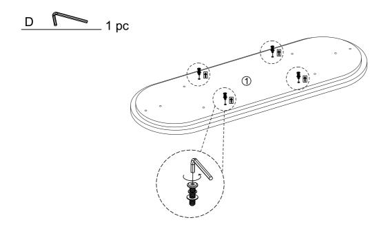
**Step 2:** Flip over the support onto the leg and attaching the support to the leg.
