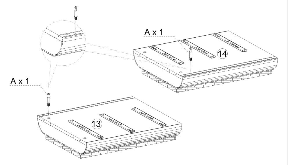
The hole with dent side should face upward
