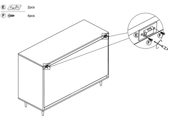
Step 4: Anti Tipping Kit Installation on the wall.
